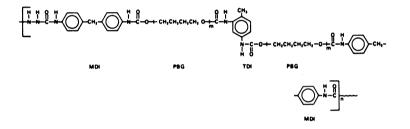
Fig. 3. Structural configuration of a segmented polyurethane (Lycra T-126).
