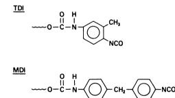
Fig. 2. Structural differences between toluene diisocyanate (TDI) and 4, 4' diphenylmethane diisocyanate (MDI).
