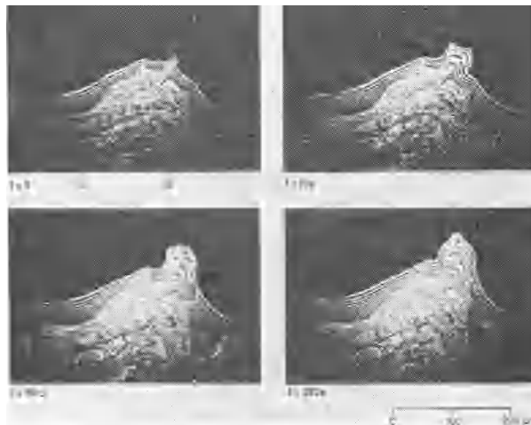
Fig. 7. Slow crack growth in partially healed material; growth occurs preferentially in zones with smallest craze band (from 20).
