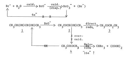
Some of these side-reactions would simply lead to a loss of current efficiency, which could be tolerated if necessary; others would leads to chemical by-products which were intolerable.
