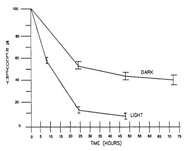
Fig. 4. Photodecomposition of Avermectin B<sub>1</sub>
