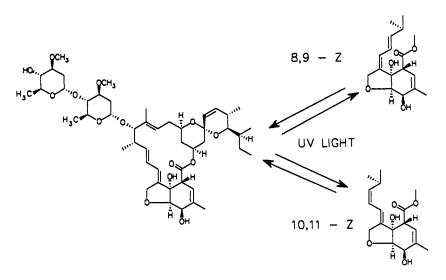
Fig. 5. Photoisomerization of Avermectin B<sub>1</sub>
