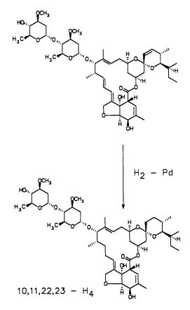
Fig. 6. Hydrogenation of Avermectin B<sub>1</sub>
