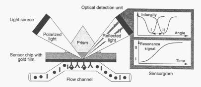
Fig. 1 Schematic illustration of the SPR detection principle.
