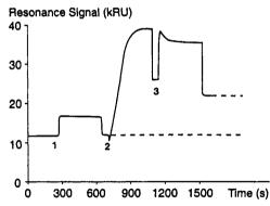
Fig. 4 Typical sensorgram of the activation and coupling of proteins under electrostatic attraction conditions: 1) activation by carbodiimide/ hydroxysuccinimide (0.2/0.05 M in water), 2) coupling of immunoglobulin G (50 µg/ml in 10 mM sodium acetate, pH 5.0), 3) deactivation of residual esters with ethanolamine hydrochloride (1M, pH 8.5).
